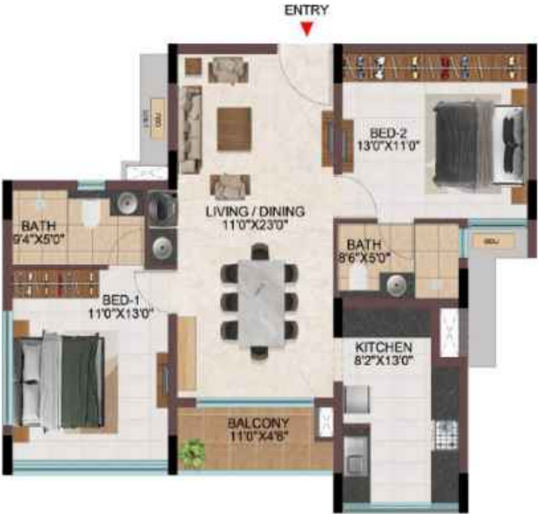
TYPICAL FLOOR ( 1 ST TO 9 TH )
