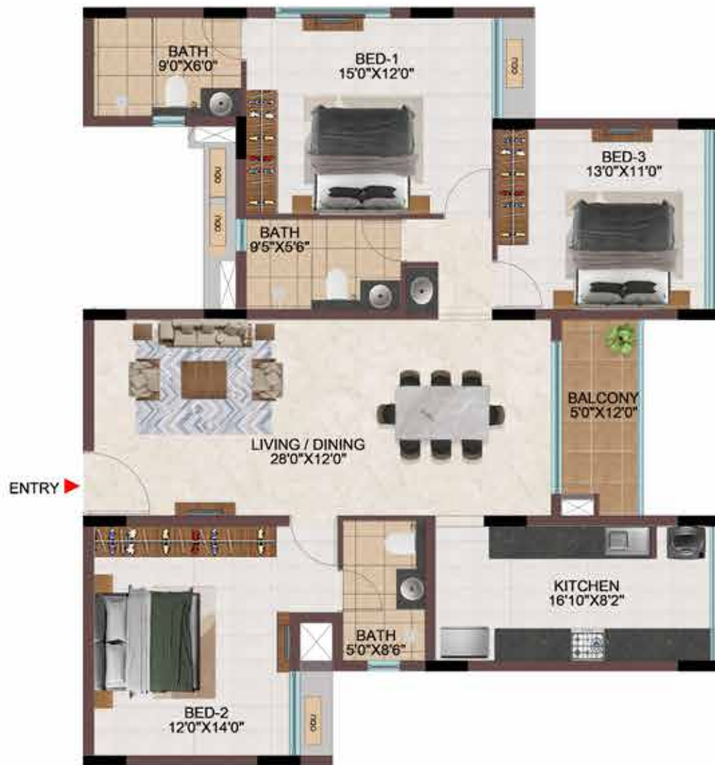
TYPICAL FLOOR ( 1 ST TO 9 TH )
