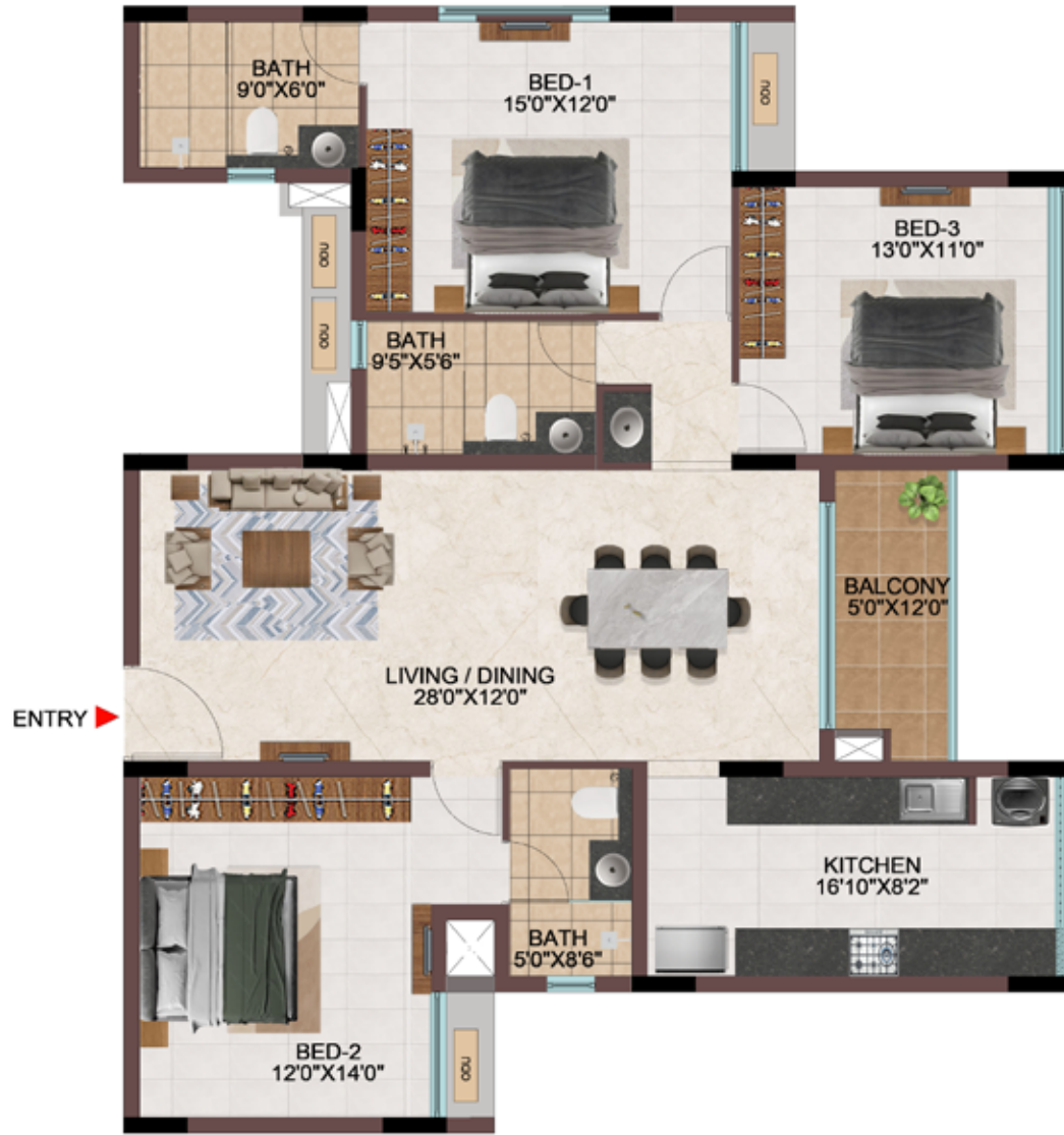
TYPICAL FLOOR (1 ST TO 9 TH )
